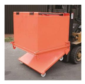
Automatic Bottom Empty Skips allow the simple but effective disposal of light to medium weight waste when being automatically emptied into high sided yard skips via the base release mechanism, without the driver leaving the safety of his seat.
